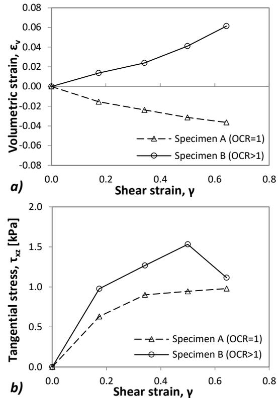
Fig. 3. a) Volumetric macroscopic response and b) mechanical behaviour of Specimen A and Specimen B upon shearing
