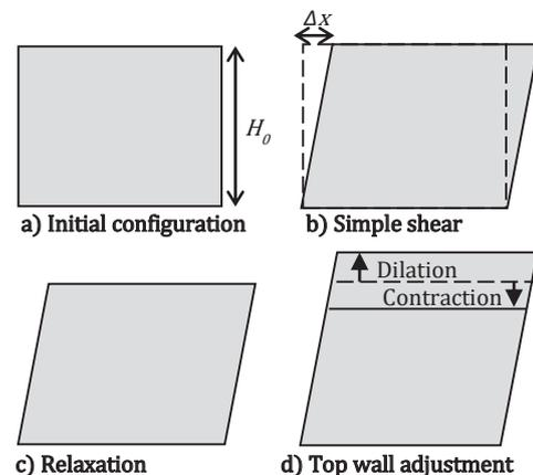
**Fig. 2.** Simulation stages for simple shear virtual experiments
