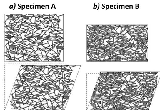
Fig. 4. Particle configuration prior to shearing (top) and after shearing to  $\gamma=0.34$  (bottom) for a) Specimen A, and b) Specimen B. Dotted lines represent the size and shape of the specimens before shearing
