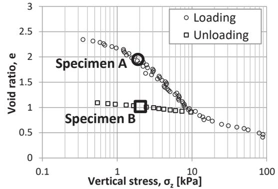
**Fig. 1.** Loading history of Specimen A (normally consolidated) and Specimen B (over consolidated) prior to shearing.
