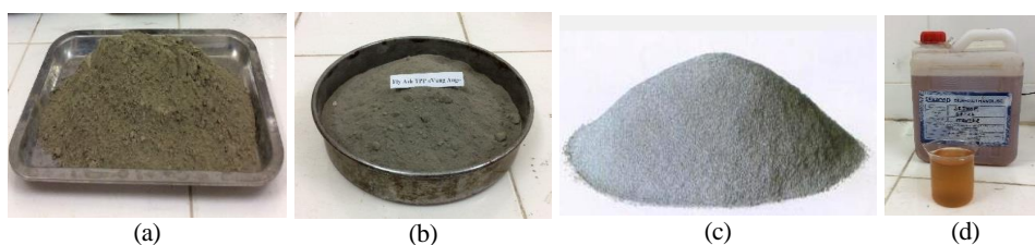
Fig. 1. (a) - Portland cement "But Son", (b) - Fly ash "Vung Ang", (c) - Aluminium powder and (d) - Superplasticizer SR 5000F "SilkRoad".
