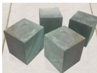
Fig. 3. The aerated concrete test specimens.
