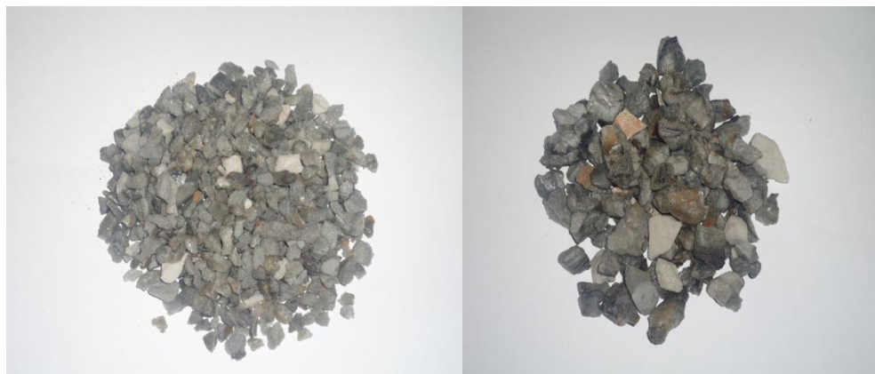
a) sizes of expanded obsidian grains: 20...10mm
