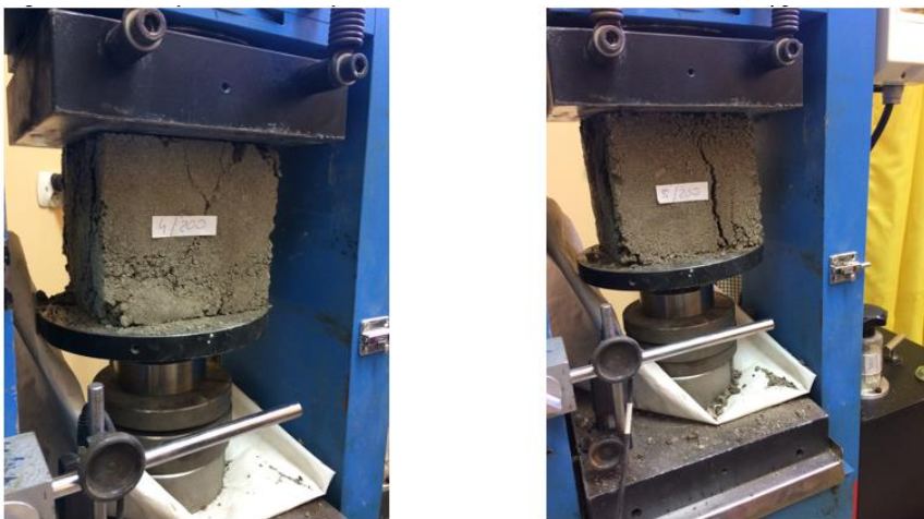
Fig. 3. and Fig. 4. Observed modes of failure mechanism in compression testing
