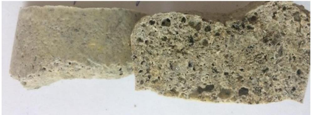
**Fig. 4.** Polymervermiculite at a weight ratio of 1: 2
