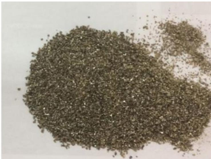
**Fig. 1.** Vermiculite swelled in the microwave
