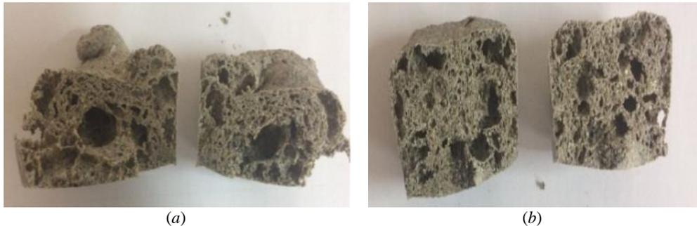
**Fig. 3.** Samples of polymervermiculite at a ratio of vermiculite: resin 1: 1 (a) and 1: 1.5 (b)
