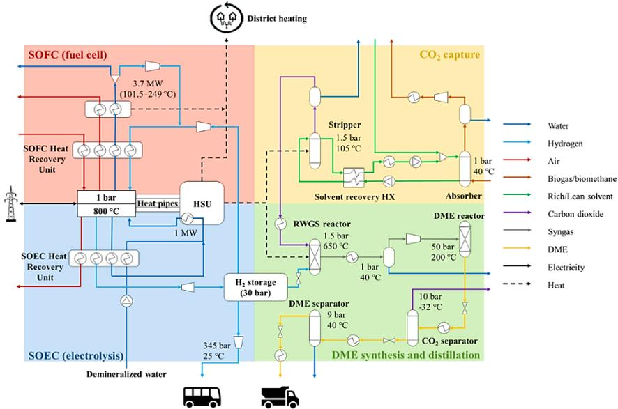
**Fig. 1.** Scheme of the ReSOC polygeneration system integrated with CO<sub>2</sub>-to-DME plant.
