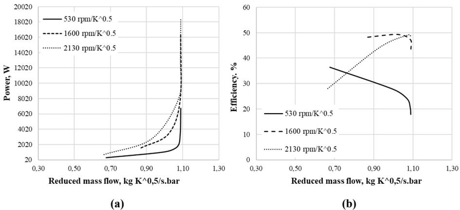
**Fig. 5.** (a) Turbine power versus mass flow rate factor for different rotational speed factors; (b) Turbine total to static efficiency versus mass flow rate factor at different rotational speed factors
