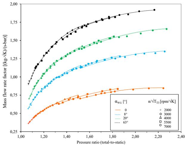
**Fig. 2.** Steady state turbocharger turbine swallowing capacity.
