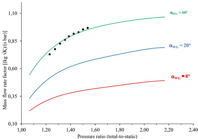
**Fig. 3.** Waste-gate valve swallowing capacity at different openings.
