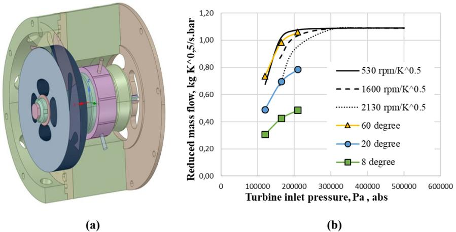
**Fig. 4.** (a) Turbine assembly cross section showing nozzles, rotor and generator in single housing; (b) Turbine characteristic curves and waste-gate valve swallowing capacity for different openings
