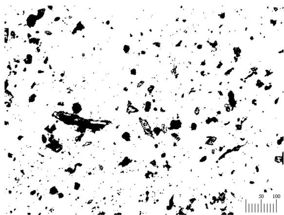
Fig. 5. The results of measurements of dust pollution of the habitable inner spaces in the building located near the construction industry in the summer and winter periods (all sizes are in mm)
