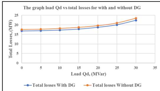
Fig. 2. The graph for load Qd versus total losses with DG and without DG.
