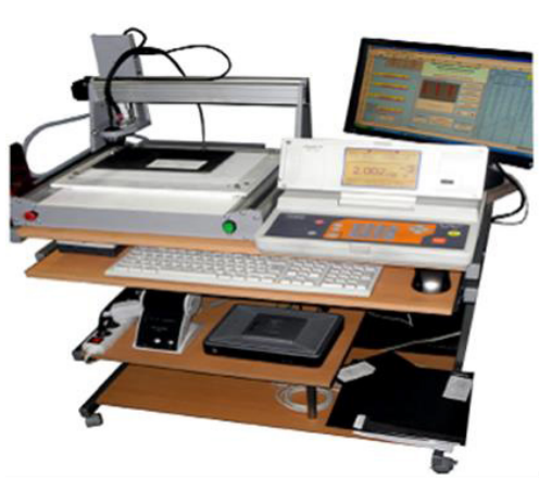
Figure 3. Testing device for electrical conductivity (in-plane) at Eisenhuth.
