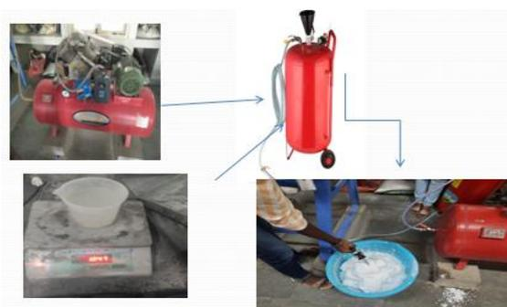
**Fig. 2.** Experimental setup for production of foam
