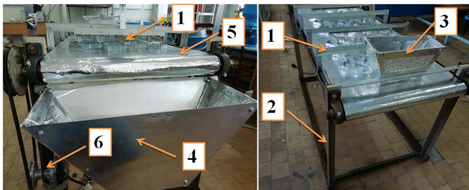
Fig. 2. Working chamber of a contact type dryer with a belt conveyor, where: 1 - casing frame; 2 - frame of the plant for drying grain; 3 - loading hopper; 4 - unloading branch pipe; 5 - conveyor belt; 6 - conveyor drive
