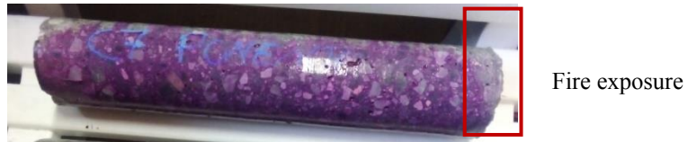
Fig. 7. Experimental tests on a concrete sample. The area in violet is representative of carbonated concrete. Total length of the carbonated zone is in the range 8 cm - 10 cm.
