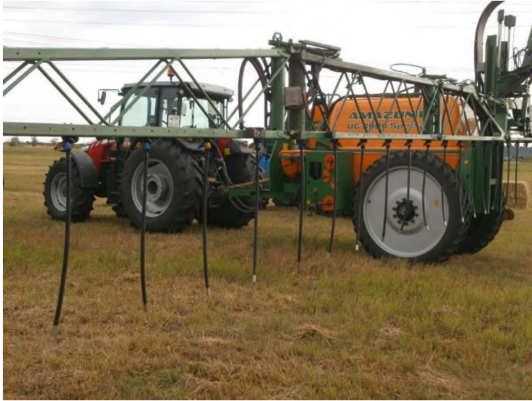
Fig. 6. Top dressing by a sprayer with extension rods
