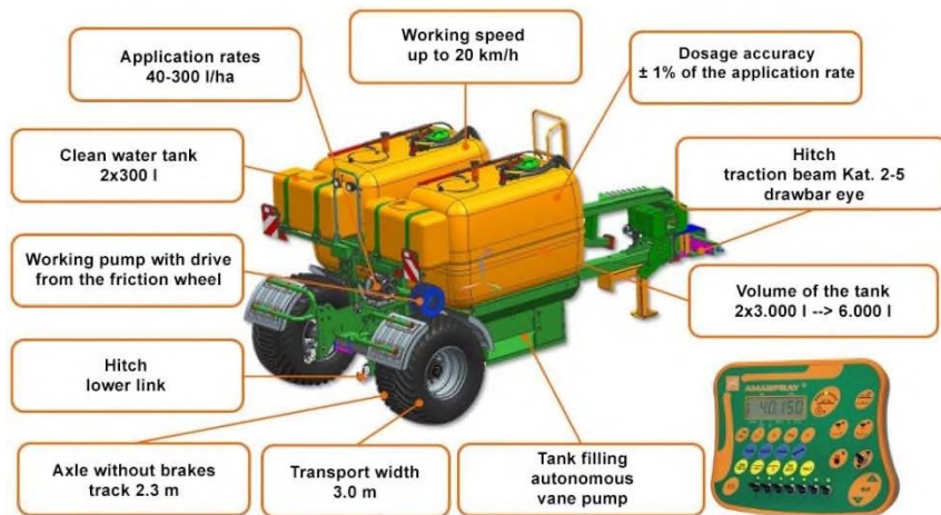
Fig. 8. Unit FDC 6000 for equipment of technological complexes – seeders of various types and purposes for the simultaneous introduction of liquid mineral fertilizers
