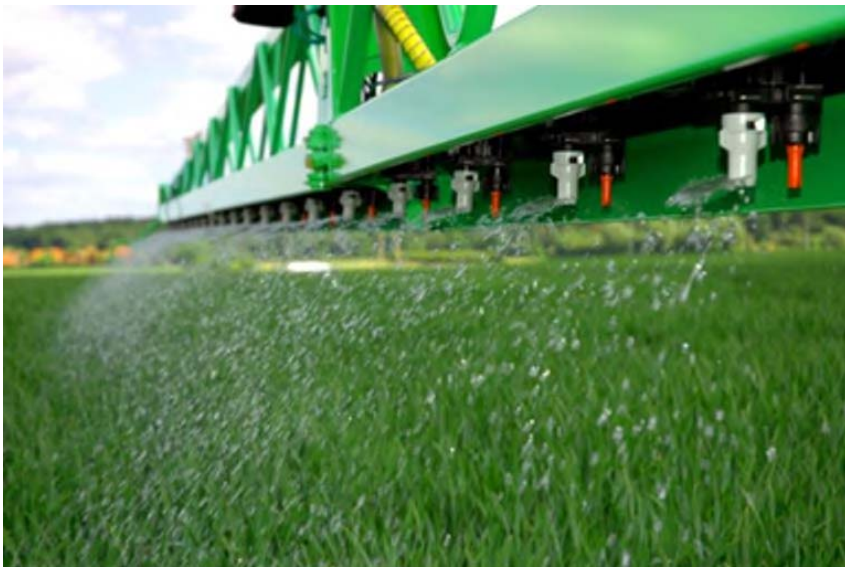
Fig. 5. Surface application of KAS by coarse droplet nozzles
