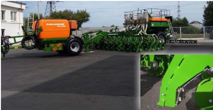
Fig. 10. Seeder DMC 9000 in unit with FDC 6000 and opener equipped with device for applying liquid mineral fertilizers
