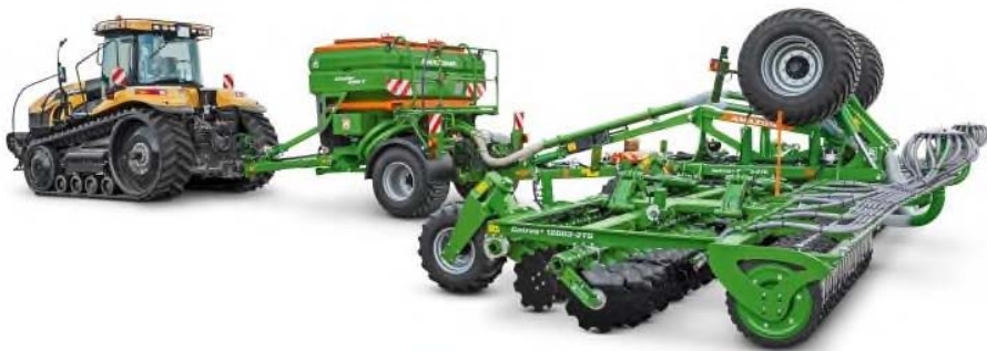
Fig. 3. Tillage and fertilizer unit: X-TenderT + Catros
