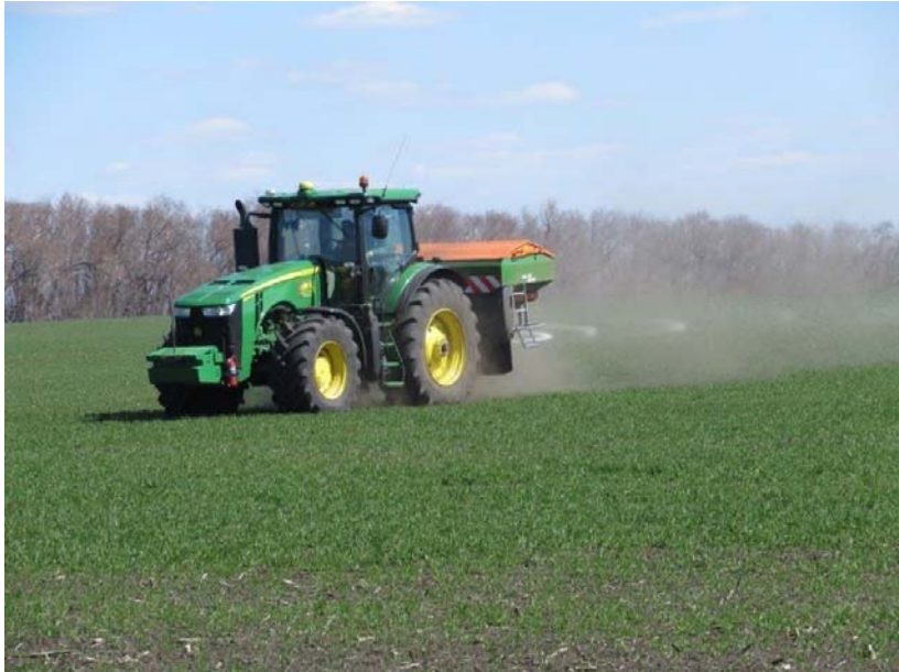
Fig. 2. Spreader of mineral fertilizers ZA-TS SamGAU in the fields of the Samara region.
