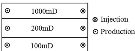
Fig 3. Schematic diagram of the 2nd planar model
