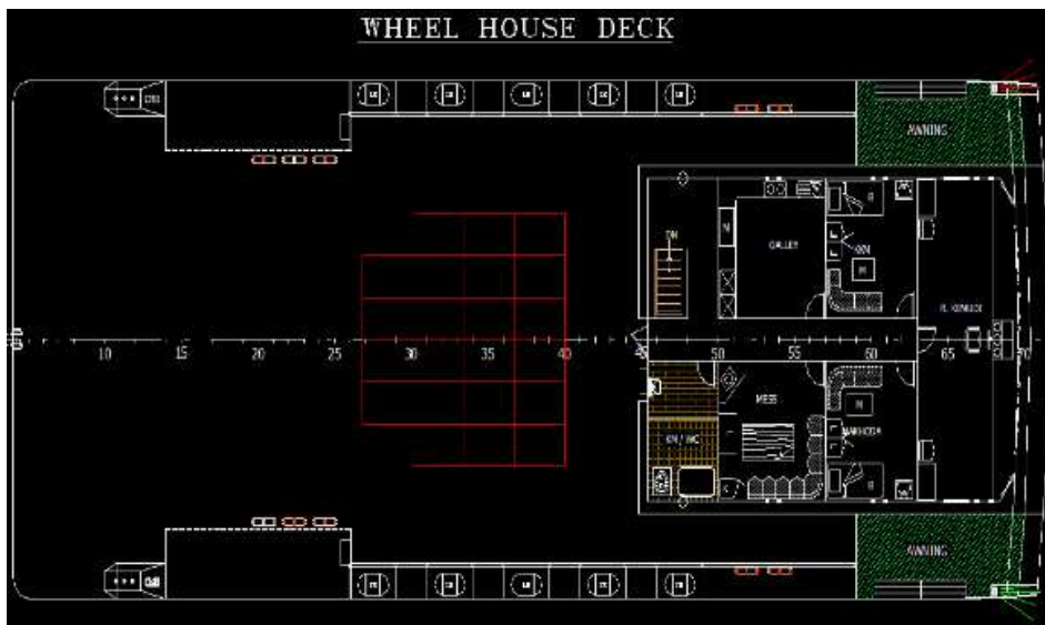
Fig. 2. The placement of solar panel in deck house
