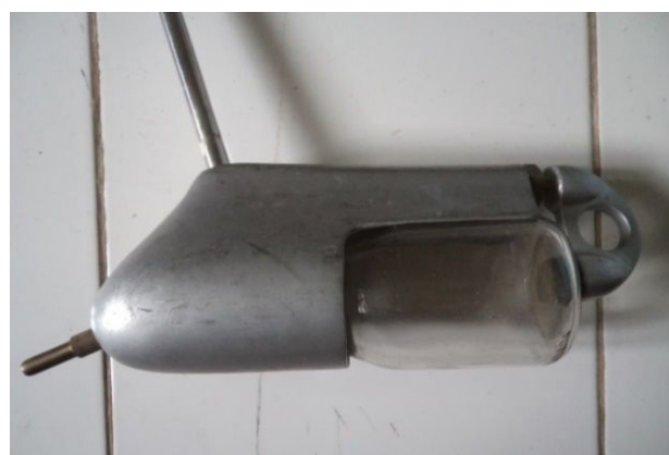
Fig. 3. Suspended sediment sampler of US DH 48 type
