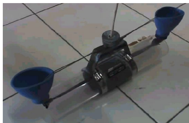
Fig. 4. Cylinder Water Sampler of LaMOTTE Model JT-1
