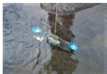
Fig. 5. Sediment sampling measurement using Cylinder Water Sampler (LaMOTTE Model JT-1)
