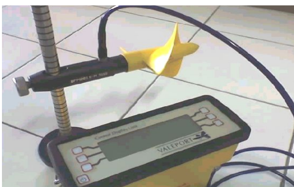
Fig. 2. Flowmeter of Valeport Model 001
