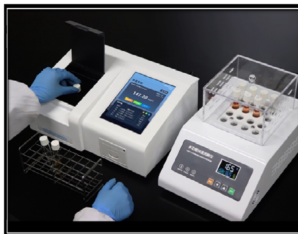
Fig.3. A picture of COD equipment (left) and thermal digestion equipment(right)
