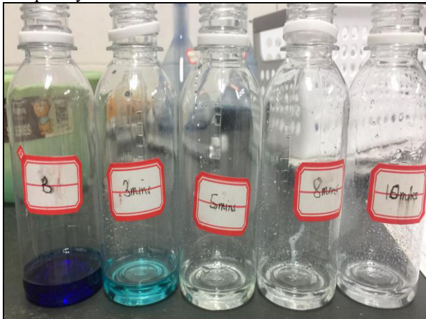
Fig.4. Decolorization effect of MB solution treated with ozone microbubble solution for 0~10min
