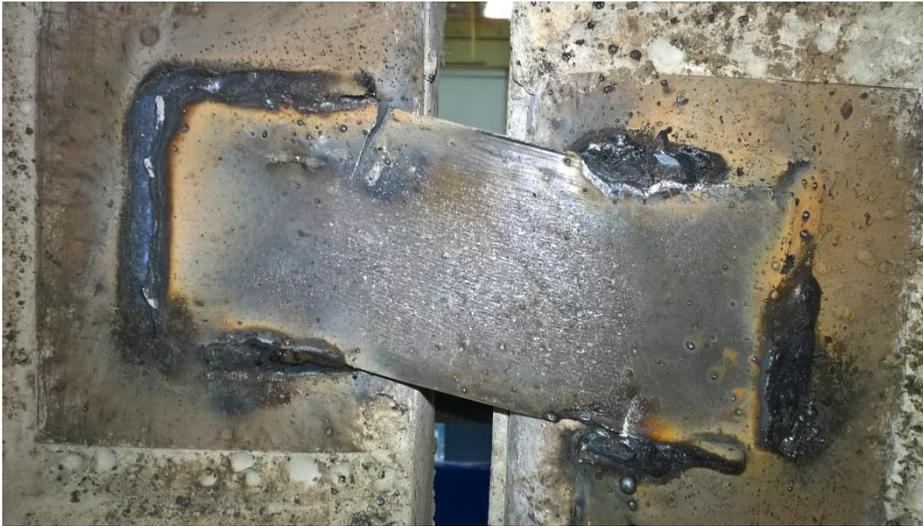
**Fig. 5.** Destruction of the connecting plate welded butt.
