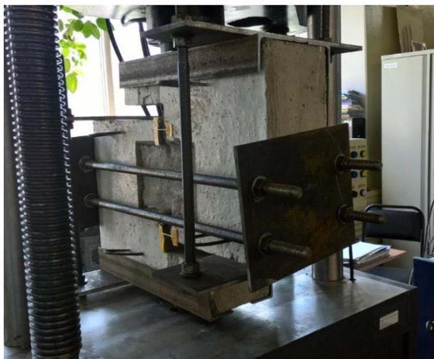
**Fig. 4.** Experimental welded butt.
