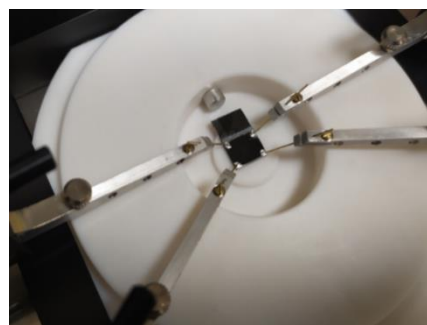
Fig. 2. Correctly installed sample in HL55PC.
