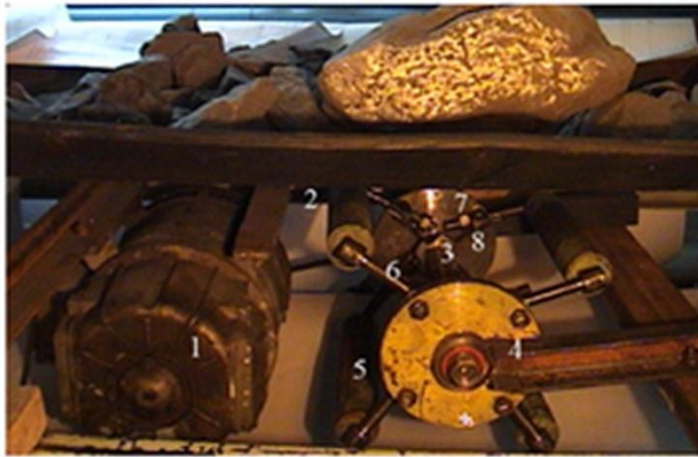
Fig. 1. Pilot unit to segregate bulk cargo by size on the conveyor belt
