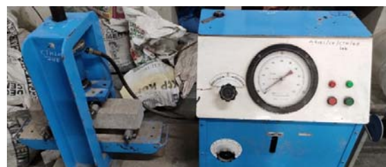
Fig. 4. Flexural strength test on prism
