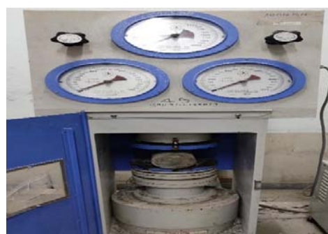
Fig. 5. Split tensile strength test on cylinder
