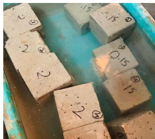
Fig 1. Water curing was done for Concrete Blocks
