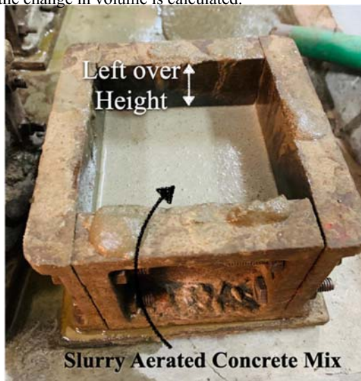
Fig 2. Left over Height of the concrete
