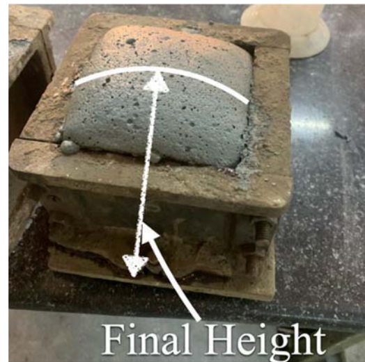
Fig 3. Final Height of the concrete
