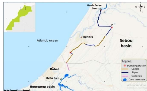
Fig. 5. Proposed scheme of the NSWTP in Morocco.
