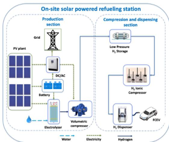
Figure 1: Scheme of the proposed on-site HRS station
