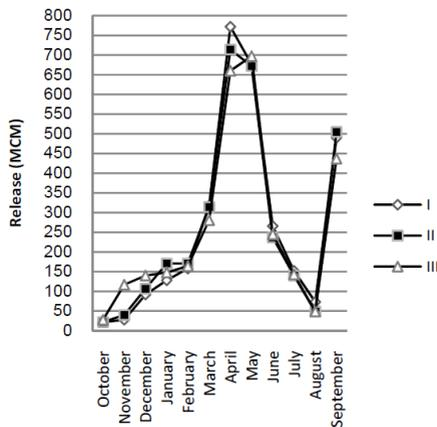
**Fig 6.** Release of Shahryar reservoir for models I, II, III
