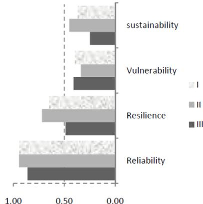
**Fig 8.** performance criteria of the Sefidrud reservoir
