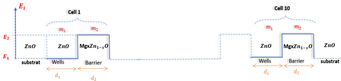
Fig. 1. Energetic profile of a MQWs constituting of 10 periods, ZnO/ Zn_{1-x}Mg_xO ( x = 0.25 ) with thicknesses equal d_1=d_2= 40\text{\AA} .
