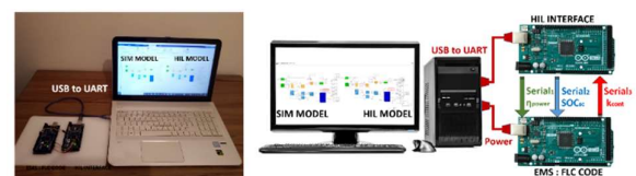
Fig. 6. Hardware-in-the-loop (HIL) architecture for proposed HESS.
