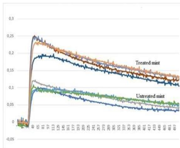
**Fig. 2.** Example of responses collected from TGS822 sensor for a day.
