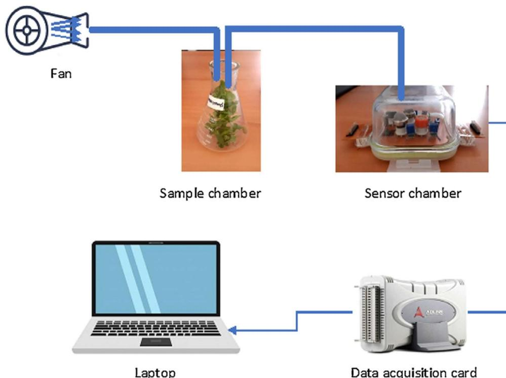
**Fig. 1** Schematically representation of the portable system utilized.
