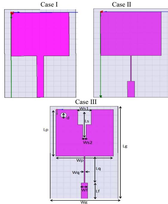
Fig. 1. Structural development stages of the basic element antenna
