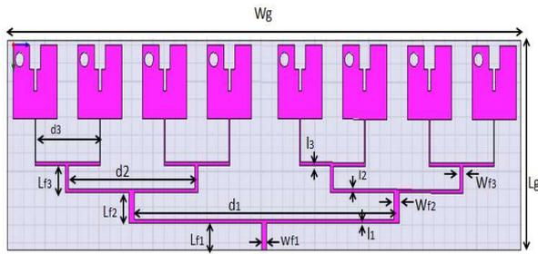
Fig 4. The structure of the proposed high gain  $1 \times 8$  array antenna
