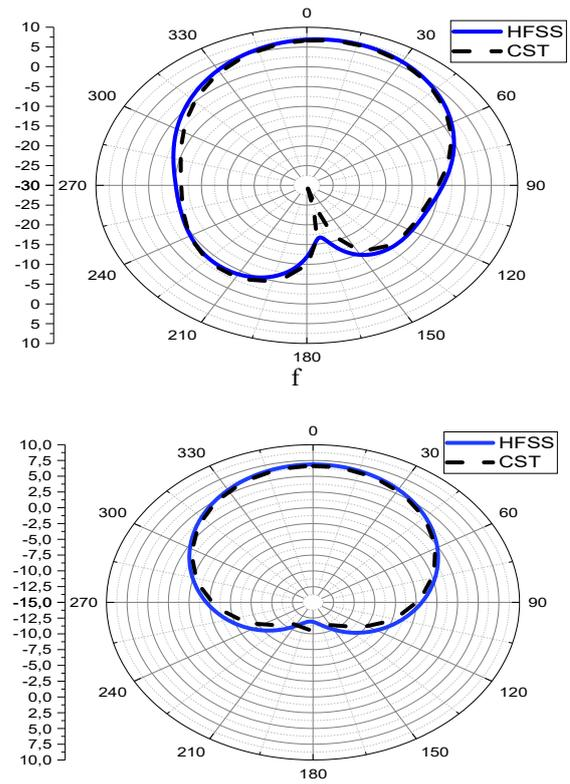
**Fig. 3.** (a) S11 parameter vs. frequency; (b) VSWR vs. frequency; (c) Gain vs. frequency; (d) Rad. Efficiency vs. frequency; (e) E plane radiation patterns at 2.4GHz; (f) H plane radiation patterns at 2.4GHz
