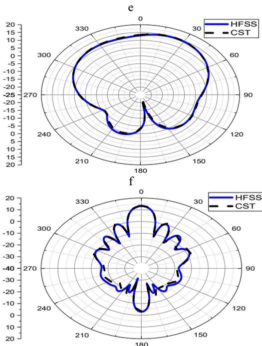
**Fig. 5.** (a) S11 parameter vs. frequency; (b) VSWR vs. frequency; (c) Gain vs. frequency (d) Rad. Efficiency vs. frequency; (e) E plane radiation patterns at 2.4GHz; (f) H plane radiation patterns at 2.4GHz
