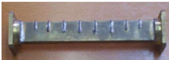
Fig 5: Prototype of a symmetrical filter formed by 8 symmetrical iris discontinuities.
