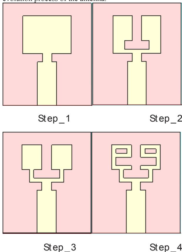
**Fig. 2.** Structure evolution for the 5G antenna
