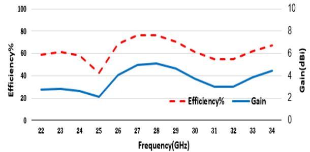
Fig. 8. Simulated Gain and Radiation Efficiency of the transparent antenna.
