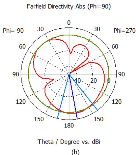
**Fig. 9.** 2-D radiation pattern of the transparent antenna (a) E-plane (b) H-plane.
