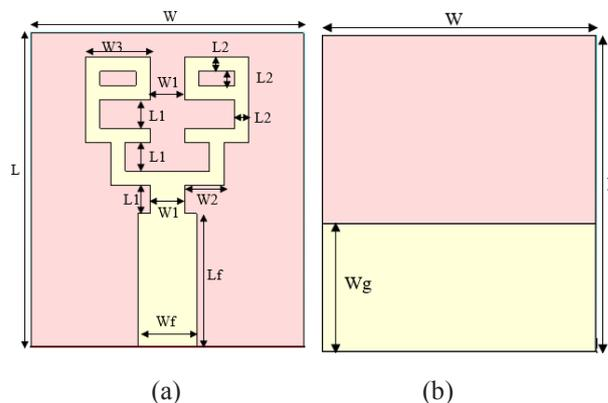
**Fig. 1.** Final Geometry of transparent antenna: (a) Front view; (b) back view
