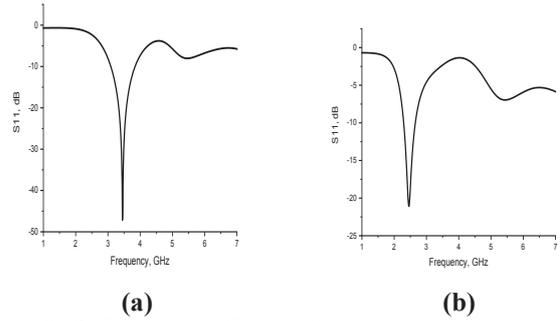
**Fig. 3.** Reflection coefficient of agile monopole antenna for two states of switch diode: (a) OFF state and (b) ON state
