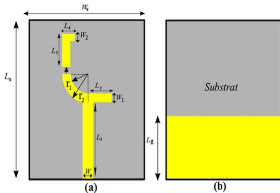
**Fig. 2.** Monopole antenna with frequency agility: (a) Front view (b) Behind view.
