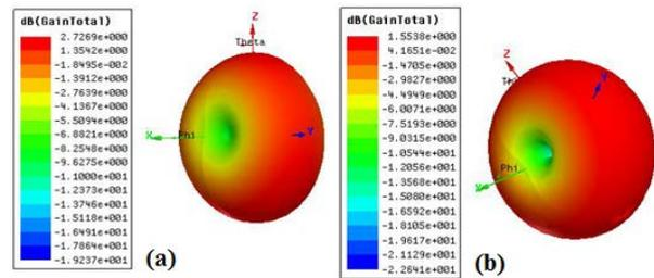
**Fig. 4.** Simulated 3D gain: (a) OFF state, (b) ON state.
