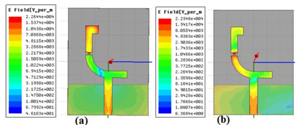
**Fig. 5.** Surface electric fields for (a) 2.45 GHz and (b) 3.45 GHz.
