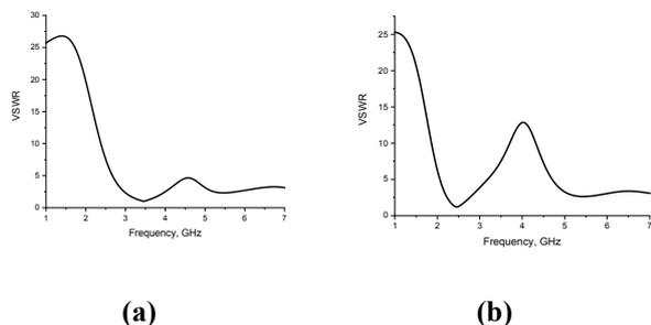
**Fig. 6.** VSWR of agile monopole antenna: (a) OFF state and (b) ON state
