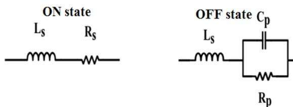
Fig. 1. Equivalent models of the switch diode in two states
