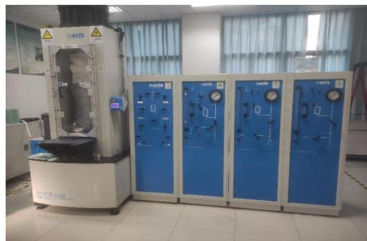
**Figure 1.** High-temperature and high-pressure rock comprehensive test system.
