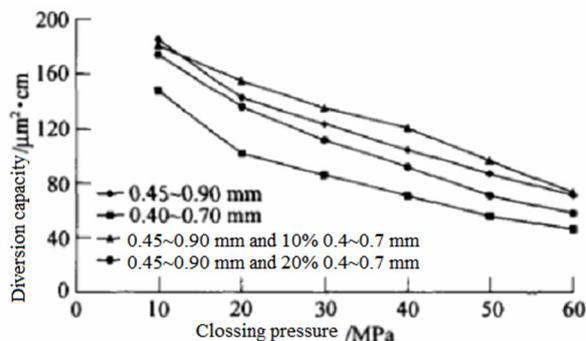
**Figure 1** Flow conductivity curve of medium density proppant
