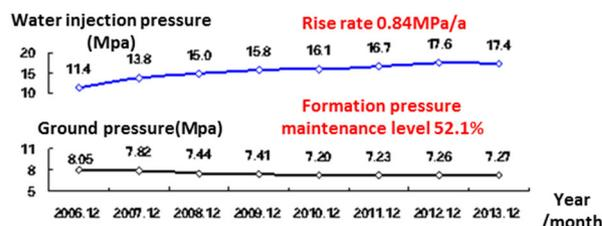
Fig.1 X oilfield water injection pressure and formation pressure variation curve
