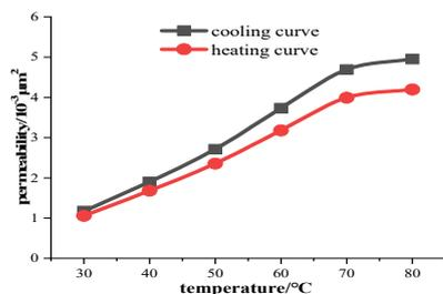
Figure 12. The permeability variation curve of No. 2 core
