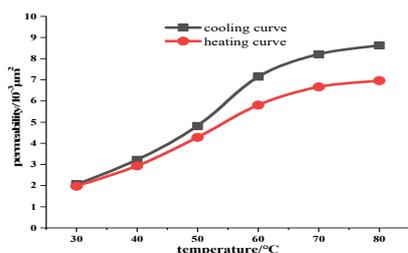
Figure 11. The permeability variation curve of No. 1 core
