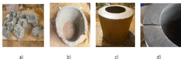
Figure 32: Steps in the manufacture of models for the removable load a) the banco, b) modeling of the hearth, c) obtaining a complete hearth, d) cutting of the hearth
