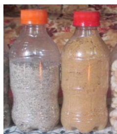
Figure.16: Jatropha cakes after mechanical (left) and traditional (right) pressing
