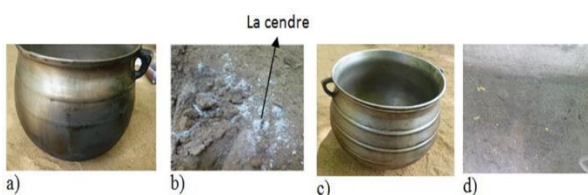
Figure 34: the level of soiling of the pots and the ground for the prototype and FABCM. a) soiling of the pot with the hearth loaded in a MINEPDED way. b) deposit of the ashes on the ground with the hearth loaded in a MINEPDED way, c) cleanliness of the pot used with the prototype, d) cleanliness of the ground with the use of the prototype.
