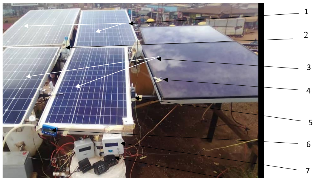
Fig.6. Hybrid PV/T water systems
