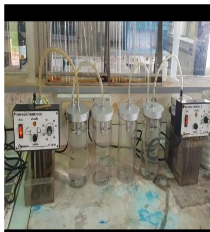
Fig.1: Biodigester and anerobic digestion
