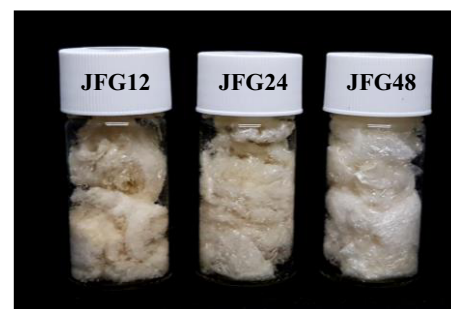
Fig. 2. Freeze-dried jellyfish by-products gelatins at various extraction times of 12 (JFG12), 24 (JFG24), and 48 h (JFG48).
