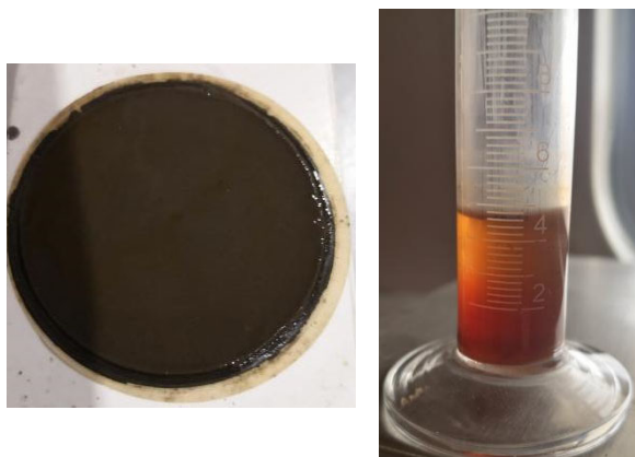
Fig.4 High temperature and high pressure for mud cake and water loss
