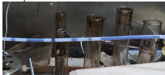
Figure 3. Air bubble method to measure the starting pressure
