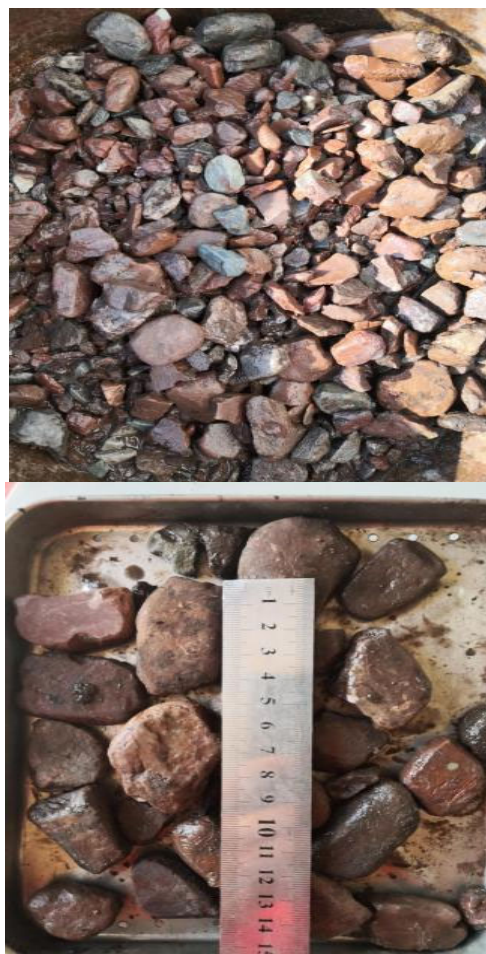
Fig. 4 Blocks returned from the pass-through of Zhong-14 well
