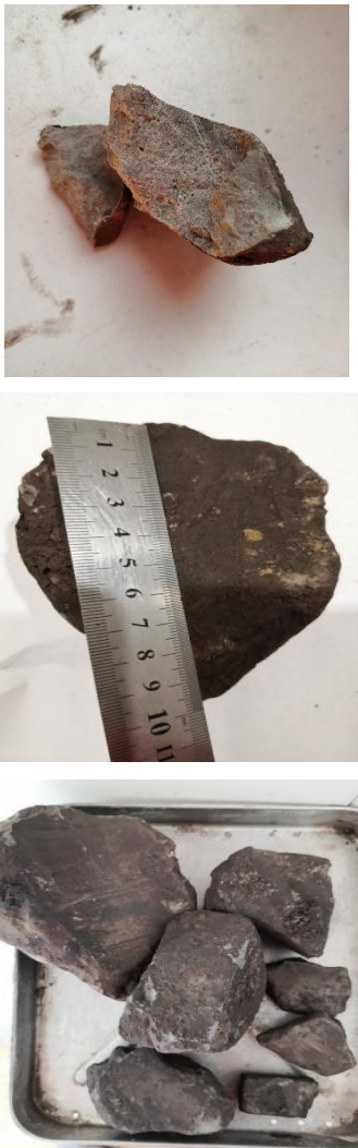
Fig. 10 The cement block returned after the first cement injection in Zhong-14 well
