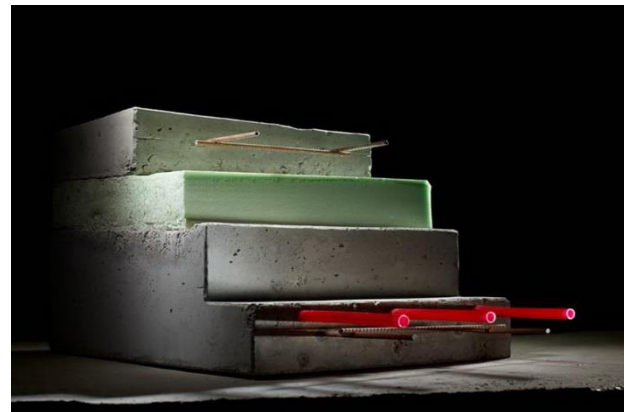
Figure 1: (Lying) cross-section of a multifunctional building part designed as an external wall.
