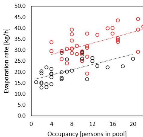
Figure 6 Scatter plot of the evaporation rate plotted against number of bathers: Black circles - Jøa; Red circles - Dalgård.
