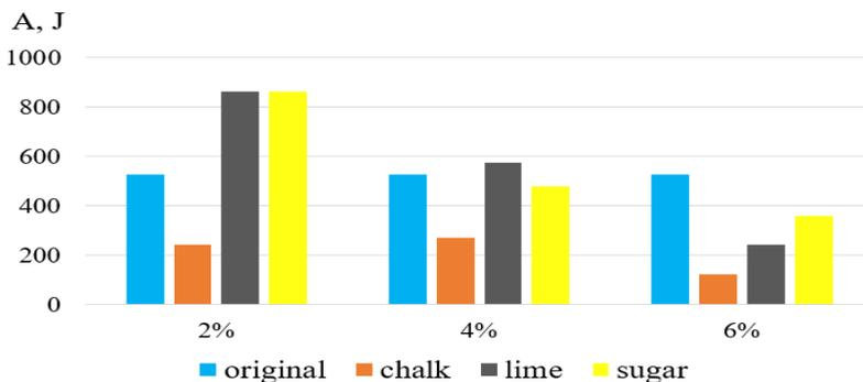
**Fig. 3.** Work expended on the destruction of samples
