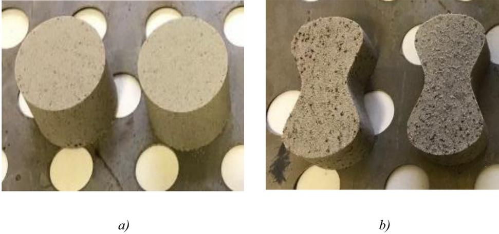
**Fig. 1.** Samples for testing mechanical properties and gas permeability, (a) and (b).
