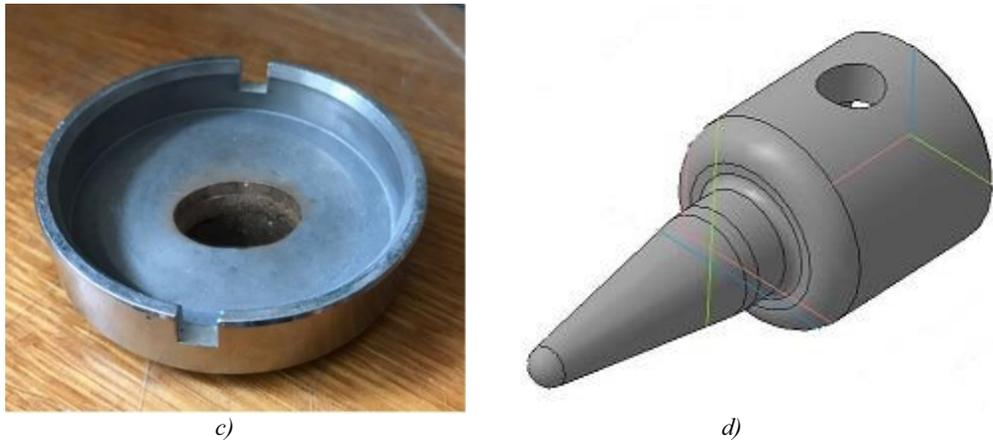
**Fig. 2.** A device for assessing the knockout of mixtures: a) is test sample; b) is metal sleeve; c) is pallet; d) is striker.
