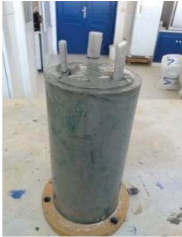
Fig.4. Insertion of three vertical drains
