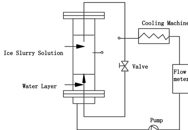
**Figure 4** Direct jet preparation of ice slurry
