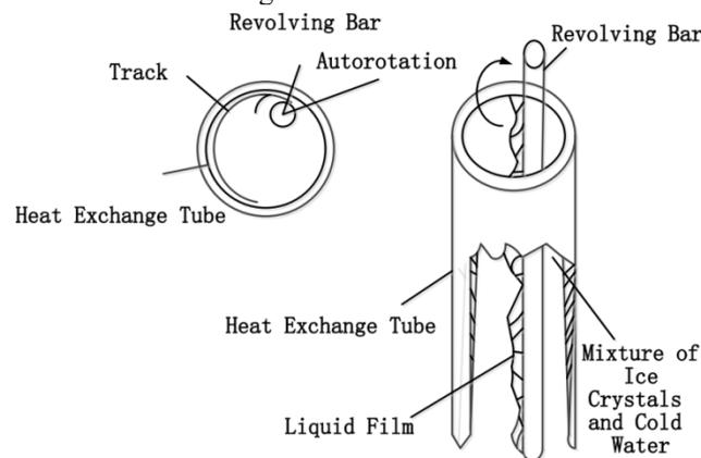
**Figure 1** The scraper ice slurry generator
