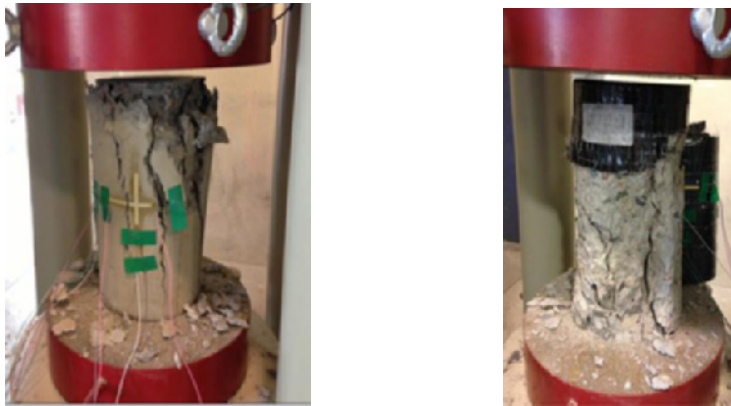
Fig. 1. Compression failure of concrete cylinders without reinforcement and with reinforcement fibro-reinforced nets.
